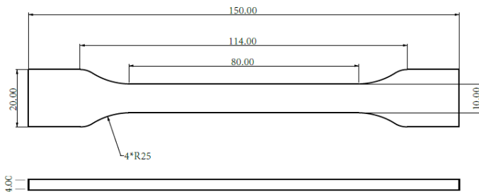
Tensile testing specimen; ASTM D638 (ISO 527, GB/T 1040)
