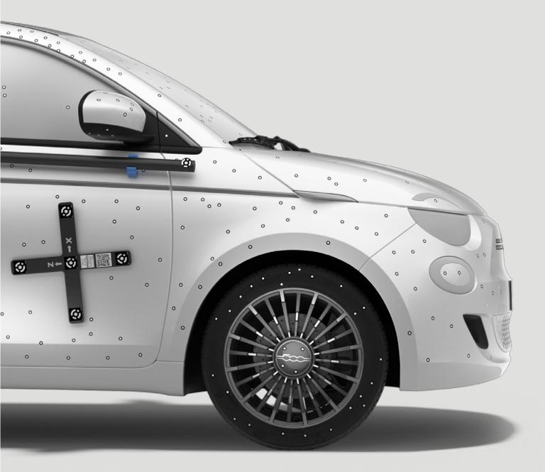
A professional photogrammetry solution with metrology-grade precision and high-end volumetric accuracy for inspection, reverse engineering, and other industrial measurement applications.
