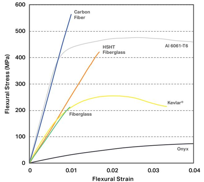
● **Carbon Fiber** Flexural Strength: 540 MPa
